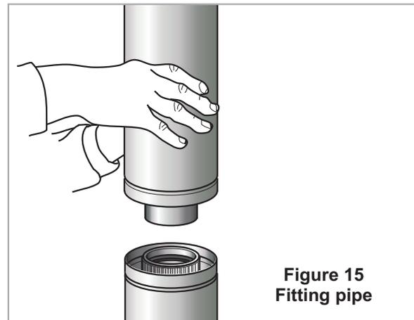
the section of flue pipe (E) in the top of section (D). The outer pipes butt together.
