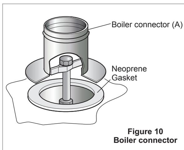
Locate the boiler connector (A) centrally into the gasket on the top of the boiler. Tighten the bolt to fix the connector in place (see figure 10).
