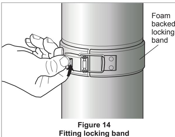
Take the fixed section (E) of flue pipe and check a red seal is in position in the swage. Lubricate the lip of the red seal in the top of section (D). Fit
