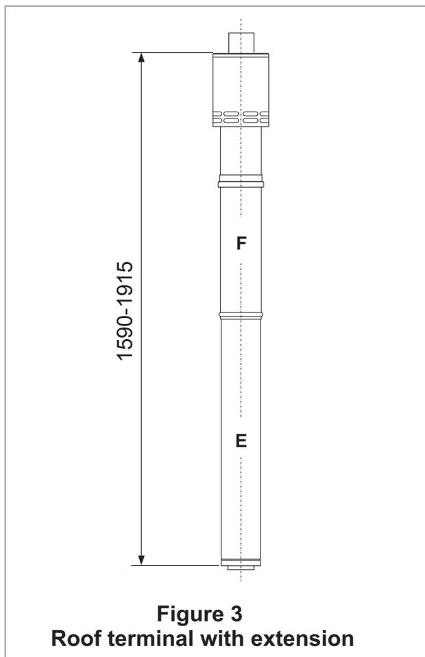
Sections (C) and (D) combine to form a telescopic length. Terminal section (F) slides telescopically over fixed length section (E).
