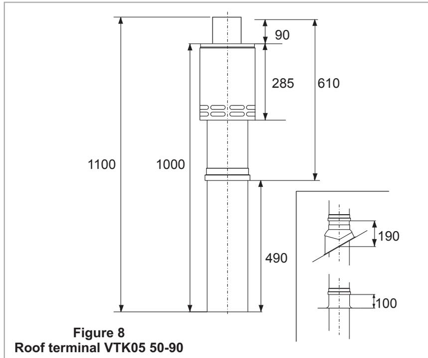
**Note:** The position of the storm collar. The storm collar locates into the top of the Grant pitched and flat flashing.
